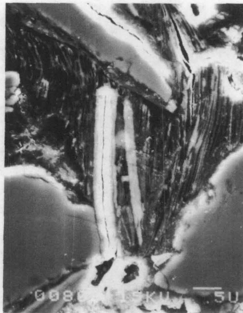
Figure VI-20. SEM Photomicrograph in Secondary Electrons of Low-Iron Chlorite Grain in Thin Section. Sample R7, Lower Member, 852 ft (258 m).
