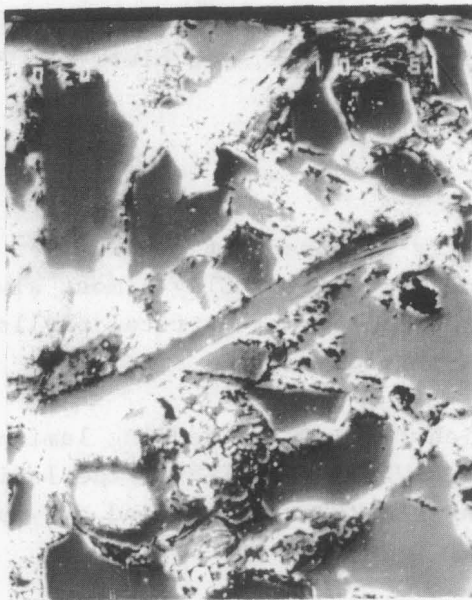
Figure VI-18. SEM Photomicrograph in Secondary Electrons of Muscovite Grain in Thin Section. Sample R8, Lower Member, 851 ft (258 m).
